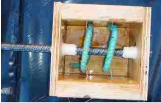
Figure 4.2 Plywood mold for pull-out specimen casting.
