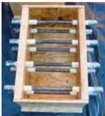
Figure 3.3 Mold to cast concrete block.
